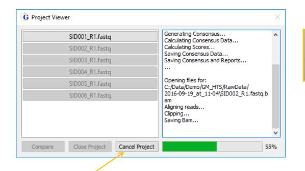
When a sample is finished it is possible to click on the button in the *Project Viewer* to open it - even before all samples finish processing
