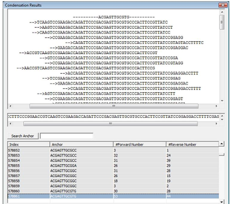
Figure 2: Condensation Results Display shows index table in bottom pane. Clicking on any index in the table displays the consensus sequence for that index above the index table with all the reads in the group shown in the upper pane lined up beneath the anchor sequence.
